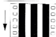
Magnetic film 35 mm 3 tracks DIN 15554 part 2 ISO 162
