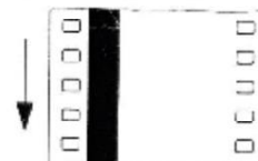
Magnetic film 35 mm Track 1 DIN 15552 part 2 ISO 162
