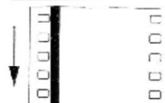
Film 35 mm with magnetic track DIN 15582
