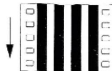
Magnetic film 35 mm 4 tracks DIN 15551 part 1 ISO 162
